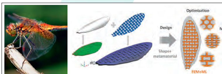
Below: Bioinspired lightweight structure for multifunctional noise control applications
