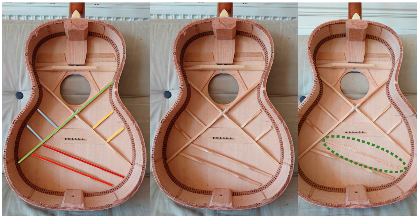
Figure 11: Soundboard bracing nomenclature (left), X-brace (green), tone bars (red), secondary tone bars (light blue and yellow). Bracing in its original state (centre) and with one tone bar removed (right). Note the large rectangular profile of all the braces
