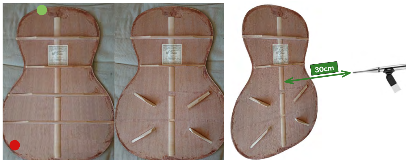
Above: Figure 16: Back with standard ladder bracing pattern (above left) and back re-worked with alternative bracing pattern similar to the one used by Gore and Gilet in 7 . In red the excitation point and in green the suspension point
