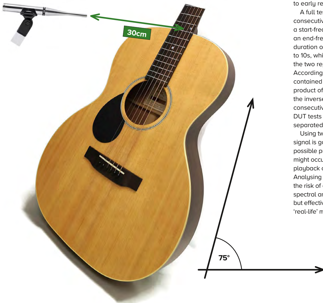
Below: Figure 7: Measurement setup. The guitar is angled at approx. 75 degrees
