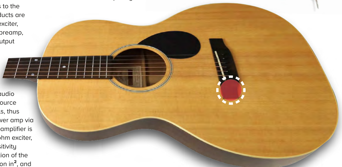
Right & below: Figure 4: A 25mm voice-coil exciter. The inner black ring is the bottom of the voice coil, which is attached to the soundboard, in yellow the spider and at the bottom the transducer's terminals. On the right, the position of the exciter on the guitar's bridge
