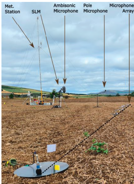
Below: Figure 1: Measurement setup, showing a 10m meteorological mast, sound level meter (SLM) for calibration, ambisonic microphone, pole microphone (at 1.5m above ground) and transversal microphone array
