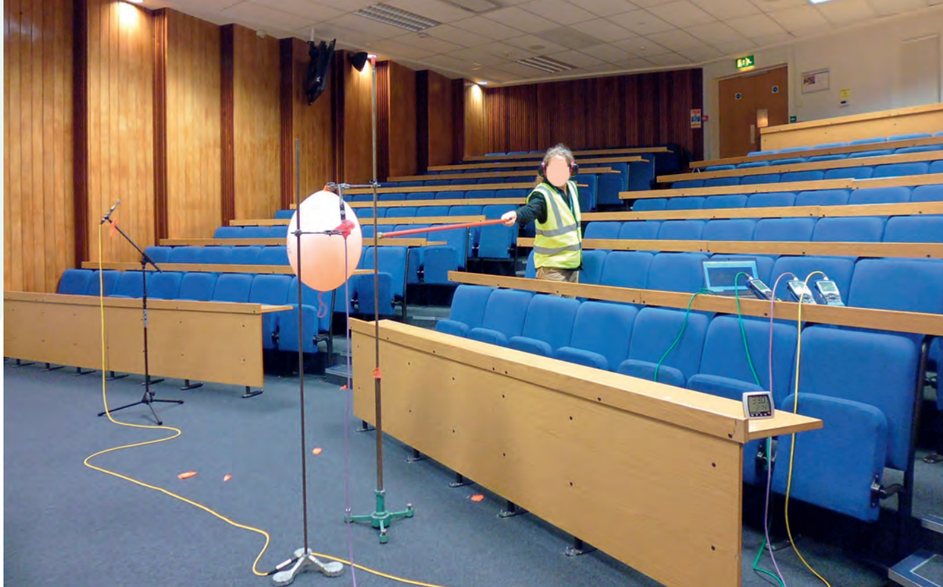
Above: Figure 2: Puncturing a large balloon at a distance during acoustic measurements in a lecture theatre
