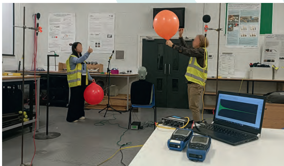
Below: Figure 1: An air-filled balloon being popped during an acoustic survey
