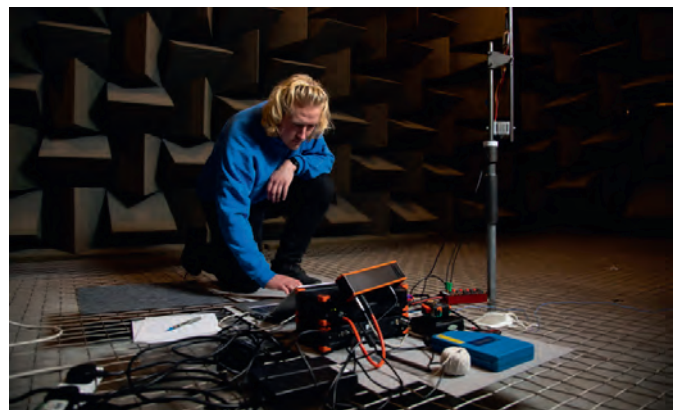
Above: Noise measurements in an anechoic chamber (image courtesy of University of Salford)
