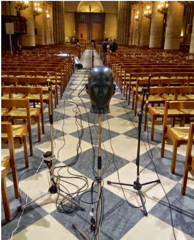
Above: Figure 2: (a) 2015, highlighting measurement equipment in the central aisle of the nave and carpet runner in a side aisle during the measurement session
