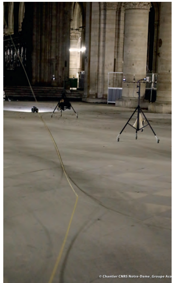
Above: Figure 2: (b) 2020, highlighting the remote-controlled robot-pulled microphone tripods and the general empty state of the nave during the measurements
