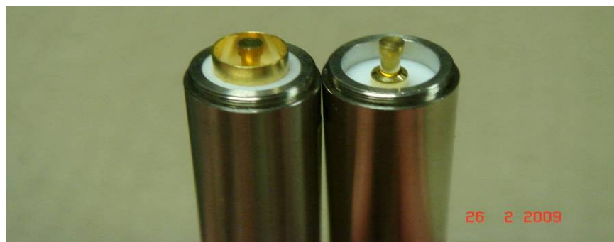
Figure 3 Preamplifier on the left has a guard ring and will have approximately 3dB better signal to noise than the one on the right
