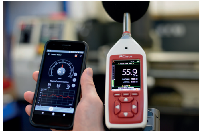
Figure 3 Comparison of a randomly selected app vs Class 1 sound level meter
