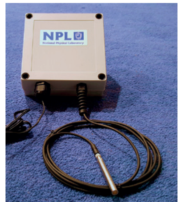
Figure 1: The NPL Raspberry Pi-based noise monitor with MEMS microphone
