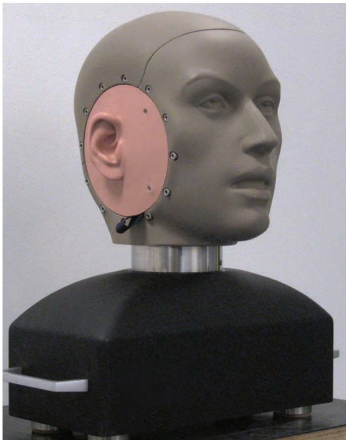
Figure 1 Head and torso simulator conforming to ANSI S12.42 (other models are available)
