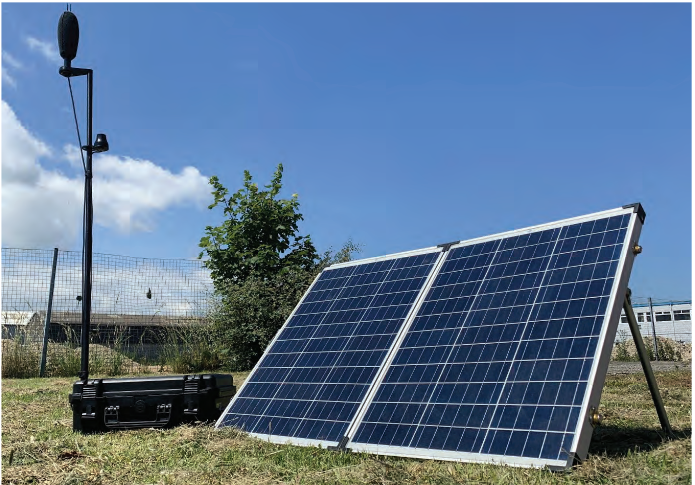
Solar powered 3G sound meter system with lead-acid backup battery
