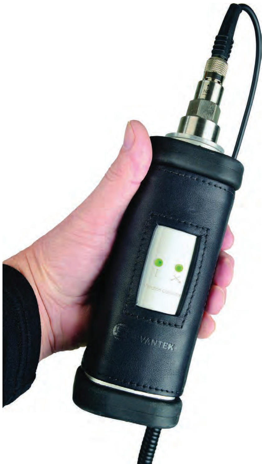
A typical hand-held vibration calibrator with preferred frequencies for hand-arm vibration
