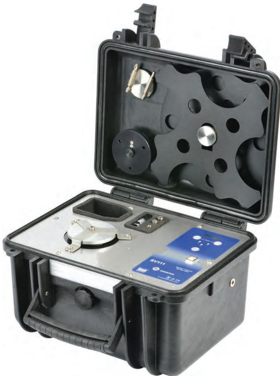
A portable vibration calibrator with preferred frequencies for ground vibration
