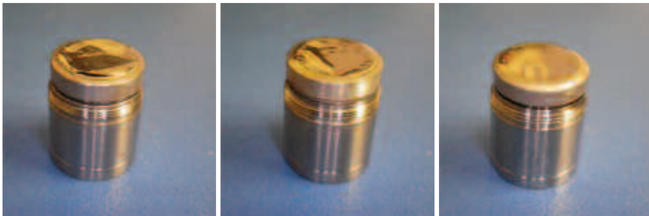
Figure 1a & 1b (left, centre): Capsules with torn diaphragms used in tests. Figure 1c (right): Capsule with obvious wrinkling, most likely caused by dropping
